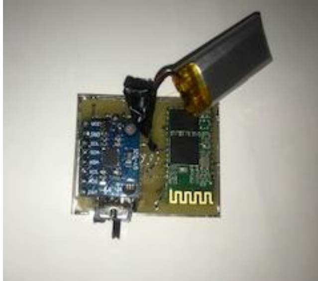
Figure 3: the developed system for measuring acceleration and angular rate of runners.
